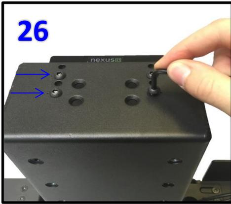
**Step 26:** Line up the “dotted” holes on the Screen Support Bracket with the “threaded” holes on the Swivel Mechanism and it using (4) 6 x 10 BHMS Screws.
