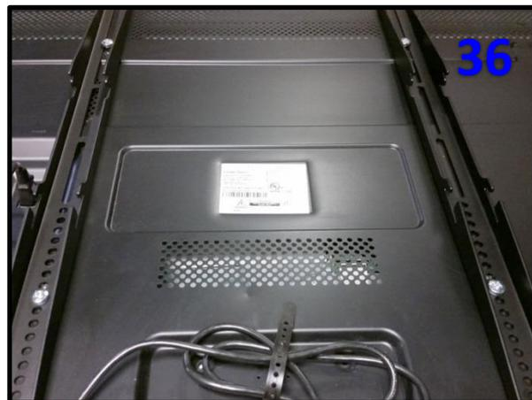
**Step 36:** Attach the Vertical Mounting Bars to the TV using the screws found in the bag labeled “TV Mounting Screws/Spacers.” The length and size of the screw required will depend on whether the TV has a flat/unobstructed or irregular/obstructed back.
