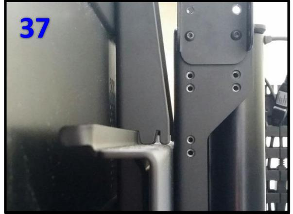
**Step 38:** Insert both *Screen Locks* into both *Vertical Mounting Bars*. Using (2) *Screen Locks*, place one *Screen Lock* on the bottom set of hooks for each *Vertical Mounting Bar*. Using a Philips Head Screwdriver (not provided), tighten the *Screen Locks* against the bottom of the *Screen Back Plate*. This will ensure the TV does not slide left to right and eliminate the TV from being lifted off of the mount.
