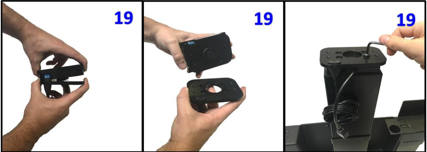
**Step 20:** Re-Attach the Swivel Mechanism to the Swivel Adapter Plate and fasten them together by tightening the screws in the unthreaded holes on the top of the Swivel.
