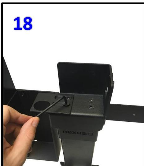
**Step 18:** Fasten the Center Riser Bracket to the Lower Actuation Assembly, then place the Right Cable Management Bracket over the first set of holes on the right side of the Upper Actuation Assembly and fasten them together using (2) 6 x 20 FHMS Screws leaving the screws slight loose. See photo to left for reference.
