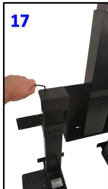
**Step 17:** Fasten the left side of the *Upper Actuation Assembly* to the *Lower Actuation Assembly* using (4) 6 x 20 FHMS Screws. See photo to the right for reference.
