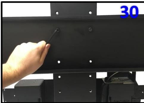
**Step 30:** Attach the *Screen Back Plate* to the *Actuation Assembly* using (2) 3/8" x 16 BHMS Screws. Mount the *Screen Back Plate* using the 4 holes towards the middle of the *Screen Support* for now as adjustments will be covered in the "**Adjustments**" section of the Instruction Manual on page (28).
