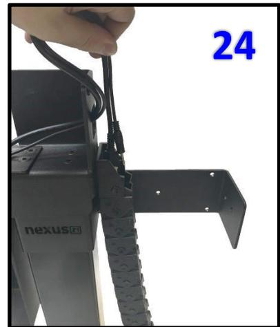
**Step 25:** Feed both the Swivel Cable and 4.5m Motor Cable through the Cable Management Track until the cables rest equal to the Lower Support Brackets.
