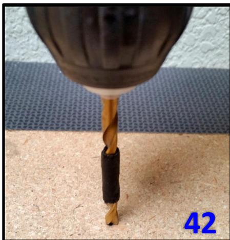
**Step 42:** Remove Cabinet Lid and drill two holes in the marked positions using a 7/32" drill bit, 1/2" deep, in the underside of the Cabinet Lid.
