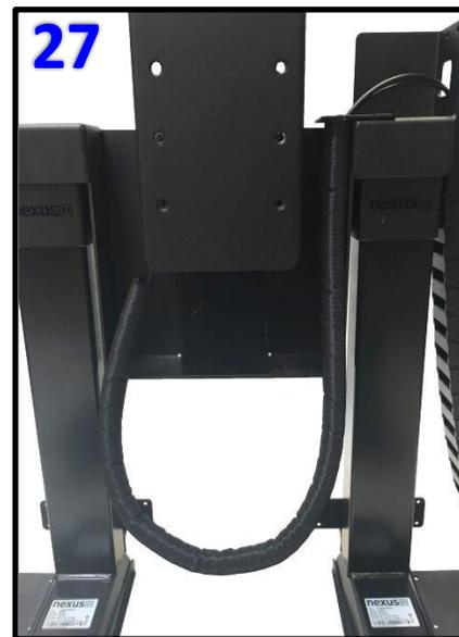
**Step 28:** Push the Snakeskin Wrap up through the Right Cable Management Bracket, slide Right Cable Management Bracket to the right the pin the cables against the Center Riser Bracket, and tighten the (2) 6 x 20 FHMS Screws.
