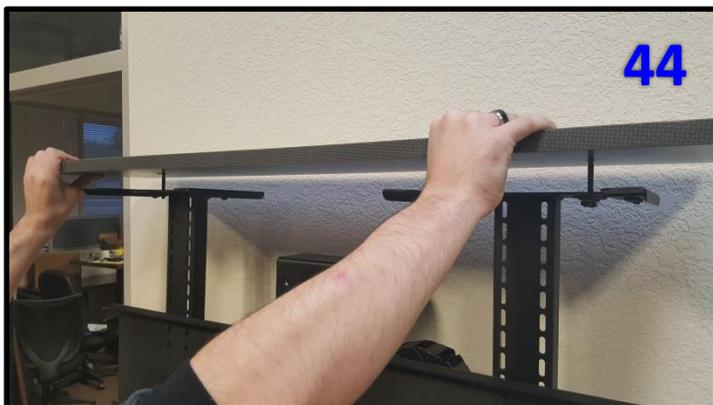
**Step 44:** Align the Tapered Pins with the holes you marked in Step 41 on the Top Plate and put the Lid on. Tighten the nuts on the underside of the hole where the Tapered Pins pass through the Top Plate.
