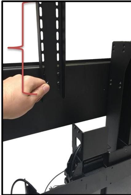
You can move the Screen Back Plate up and down, along the Screen Support to raise and lower the position of the TV on the lift. See photo to the left for reference.
