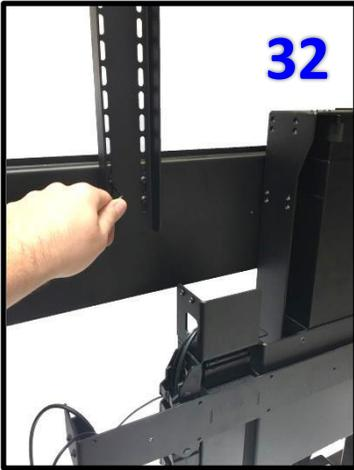
**Step 32:** Attach both of the *Top Plates* to the top of the *Top Support Brackets* using (4) 6 x 12 FHMS Screws. Ensure that wings of the *Top Plate* are pointing towards the front of the Lift System. See photo to the left for reference.
