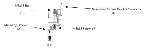
3. Insert chains (not included) through the loop holes of the **Suspended Ceiling Bracket Connector**(D).
