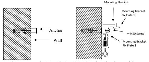
3. Attach the screen to the **Mounting Brackets (A)** by inserting the top of the case to Fix Plate 1 and securing the back of the case to Fix Plate 2. Make sure the case slots are securely attached to the mounting brackets.
