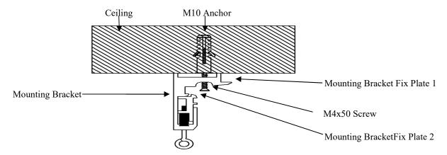
3. Attach the screen to the **Mounting Bracket (A)** by inserting the top of the case to **FixPlate 1** and securing the back of the case to **Fix Plate 2**. Make sure the case slots are securely attached to the **Mounting Bracket (A)**.
