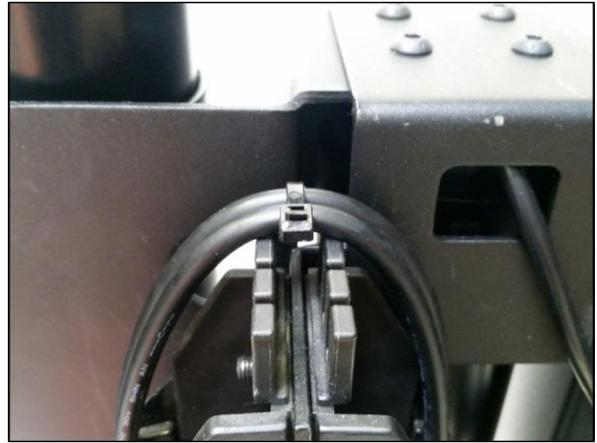
**Step 17:** Connect the *Lower Cable Chain* to the *Lower Cable Chain Bracket*. Using (2) 5mm x 12mm FHMS Screws attach the *Lower Cable Chain* to the *Lower Cable Chain Bracket*. Once connected continue routing the upper *Motor Cables* through the lower *Cable Chain*.
