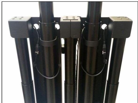
**NOTE:** Place a *Zip Tie* around the lower three 2.5 Meter *Motor Cables* and a *Zip Tie* around the upper two 4.5 Meter *Motor Cables*. This will aid in identifying which *Motor Cables* go to which *Lift Columns*. It is critical to not mix up the *Motor Cables* and accidentally plug the upper *Lift Columns* into the same *Control Box* as the lower *Lift Columns*.
