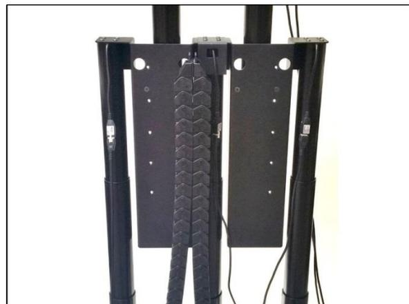
**Step 14: Attach the upper Cable Chain to the Upper Cable Chain Bracket.** Lower the upper Lift Columns, so the Upper Cable Chain Bracket is accessible. Using (2) 5mm x 12mm FHMS Screws fasten the upper Cable Chain to the Upper Cable Chain Bracket. The Cable Chain will bend into a U-Shape.
