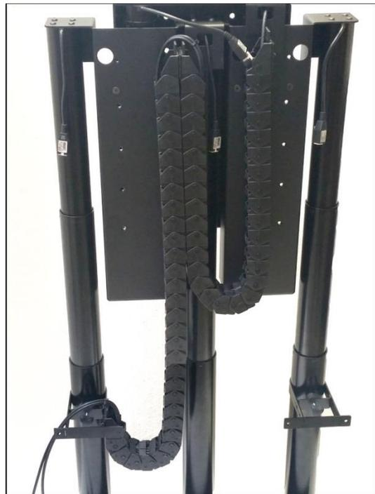
**Step 18a: Route the lower right 2.5 Meter Motor Cable through the lower Cable Chain.** Route the Motor Cable through the hole on the Column Support Bracket. Next, slide the Motor Cable through the Wire Clips on the inside walls of the Column Support Bracket (previously install in step 5). Then route the Motor Cable through the second hole on the Column Support Bracket. Last, route the Motor Cable through the lower Cable Chain.
