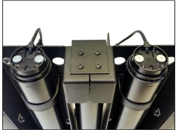
**Step 8: Temporally connect both upper *Lift Column B's* to the *Control Box (Part #8)*.** Connect the two 4.5 meter *Motor Cables* to the pigtails of the two upper *Lift Column B's* and connect the *Control Box* and *IR or RF Controls* (depending on which controls you ordered) as shown in the wiring diagrams on pages 14 and 15.
