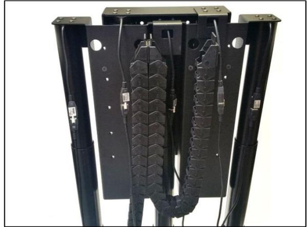
**Step 15: Route the upper two 4.5 Meter Motor Cables through the upper Cable Chain:** Extend the upper two Lift Columns, as this will aid in routing the Motor Cables. Disconnect the two upper Motor Cables from the Control Box and route each cable down through the Cable Chain.
