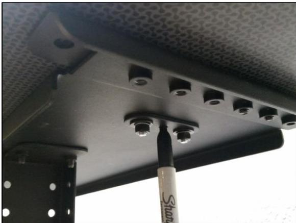
**Step 32a: Drill two  $\frac{1}{2}$ ” deep holes into the bottom side of your lid.** Using a  $\frac{7}{32}$  Drill Bit (not provided) drill two  $\frac{1}{2}$ ” holes into the bottom side of your lid in the marked positions from the previous step.
