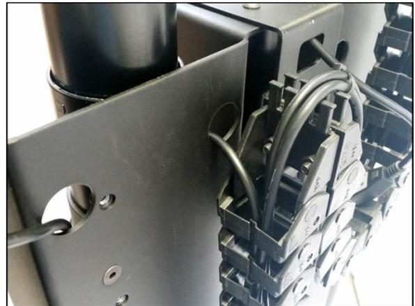
**Step 18b: Route the lower center 2.5 Meter Motor Cable through the lower Cable Chain.**
