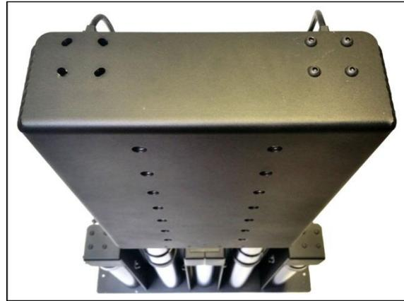
**Step 10b: Fasten the Upper Chain Bracket (Part #15) to the Screen Support (Part #4).** Align the four holes on the Upper Chain Bracket with the four holes on the Screen Support and the four threaded holes on the top of the Lift Column. Using (4) 6mm x 16mm BHMS Screws fasten the Upper Chain Bracket and Screen Support to the top of the left upper Lift Column.
