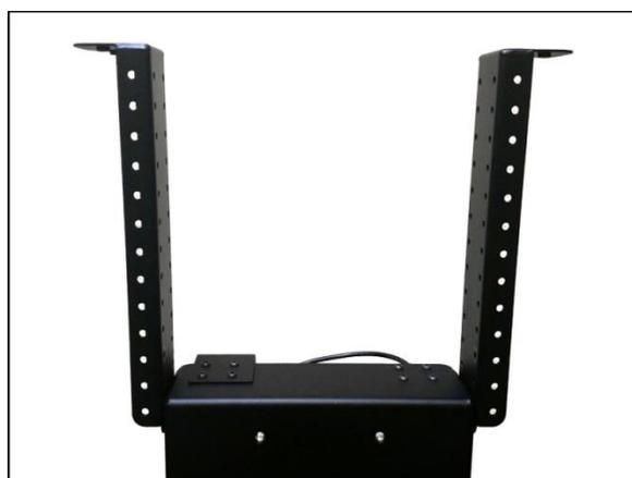
**Step 20: Attach the *Top Plate (Part #5)* to both *Top Support Brackets*. Using (4) 6mm x 12mm FHMS Screws fasten the *Top Plate* to the top of the *Top Support Brackets*. The four countersunk holes on the *Top Plate* are offset, make sure to position the edge closes to the four countersunk holes towards the front of the lift.**
