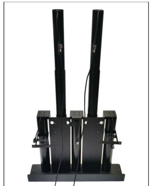
**Step 10a: Attach the Screen Support (Part #4) to the upper right Lift Column.** Using (4) 6mm x 16mm BHMS Screws fasten the Screen Support to the right upper Lift Column. Do not attach the left upper Lift Column, as this will be performed in Step 14b.
