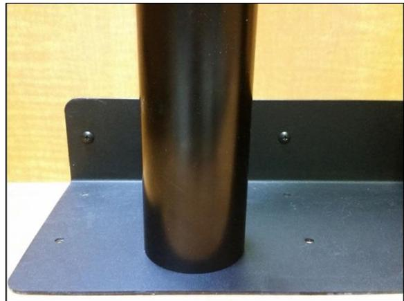
**Step 25b:** Attach the *Base Mount* to the top of the platform or base of the enclosure: Using (8) #10 x 3/4" *Truss Head Wood Screws* fasten the *Base Mount* to the top of the platform or base of the enclosure.
