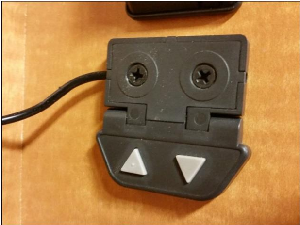
Wired Back Up Switch
