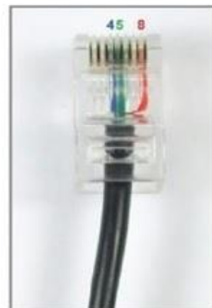
Close-up View of RJ-45 Pins
