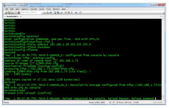
After rebooting, switch will run configuration file C2960-JPX.cfg.
