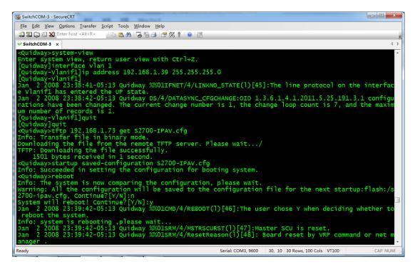
After rebooting, switch will run the configuration of S2700-JPX.cfg.
