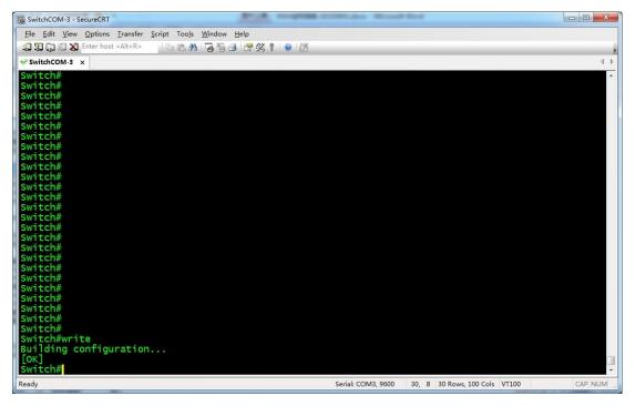
Now, it has successfully saved configuration used in single switch networking. Switch will run this
